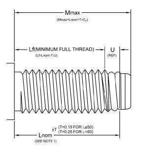
FINISHED PART DIMENSIONS Z<sub>5</sub>, Dx, & U MUST NOT BE USED TO DESIGN THE BLANK!
